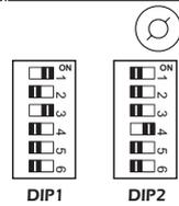
Fig. 6. To select timing at 1h. and 45 min.
