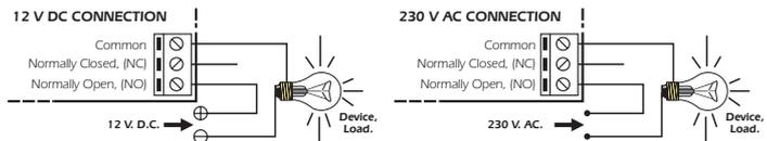
**INFORMATION ABOUT THE OUTPUT.** During the operating mode and according to its load, it could happen a fluctuation or an incorrect working of the output. In such case, you have to install an anti-spark circuit between both contacts of the used relay, as it is indicated on the schedule.
