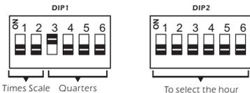
**On DIP2, only one switch has to be in ON position. If there were several switches on the ON position, or if all switches were in OFF position, the module would identify the selection as wrong and wouldn't start the timing.**
