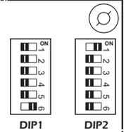
**Note.** To allow the module to recognise the timing value change on DIPs, you have to reset the circuit. Disconnect the power supply and then make changes. Finally, connect again the power supply.
