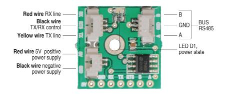
To offer the best flexibility, all the lines (power supply, RX, TX, serial TTL RTS, RS485 A and B) are replicated to the side board areas and to the pin-strips, making it easy to plug on other boards.
