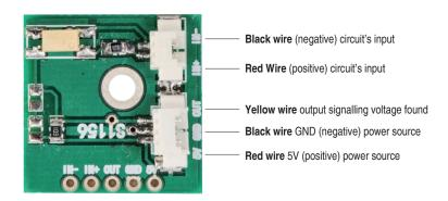
The photocoupler's input LED will be turned on even by quite feeble currents: on the order of a milliampere. The C.T.R. (Current Transfer Ratio), that is to say the ratio between the output current (in this case it is the phototransistor's collector current...) and the input current is
