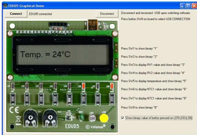
When you switch on the “Show binary value of button pressed” option, the PC screen and board will indicate the binary value of the clicked button. In the example above button 5 was clicked.
