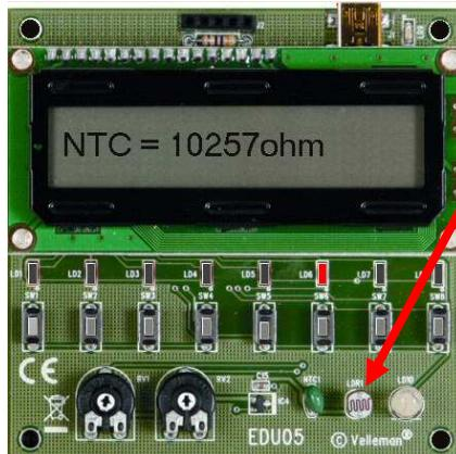
This shows you the value of the temperature dependent resistor (NTC).
