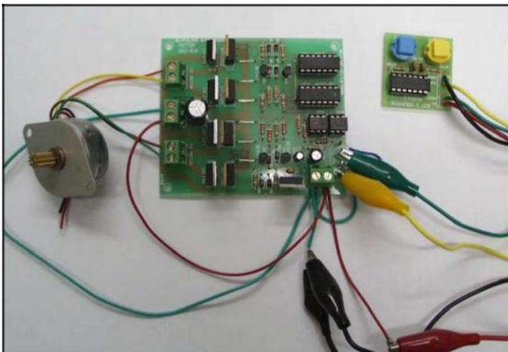
We used the debounced Counter Module of our Kit 3001 to test Kit 3158. You can get the schematic for it here [quasarelectronics.co.uk/kit-files/3000/3001.pdf](http://quasarelectronics.co.uk/kit-files/3000/3001.pdf)
