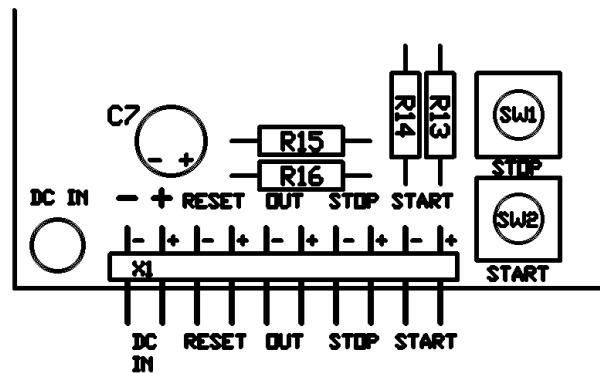
The ‘+’ sign indicates the actual input or output pin and the ‘-’ sign indicates its associated ground pin.
