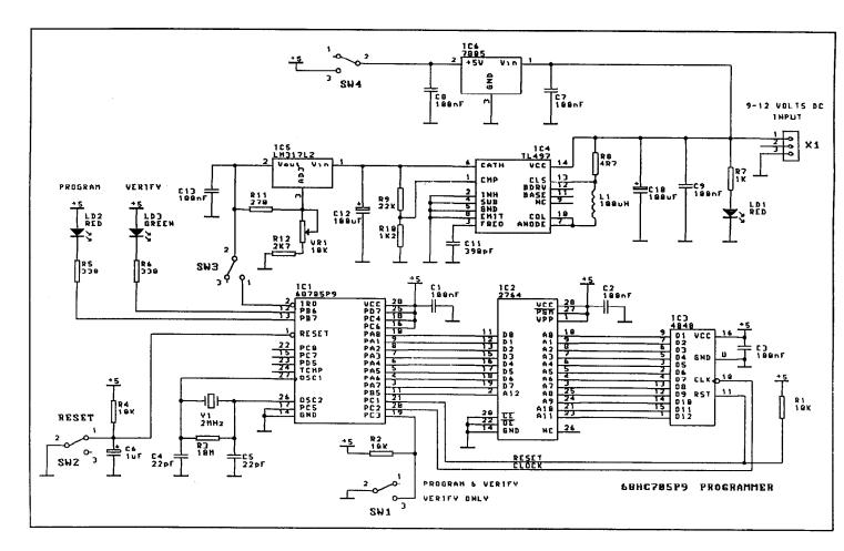
1. Connect a 12 volt DC regulated power supply via jack X1. Led LD1 should light up.
